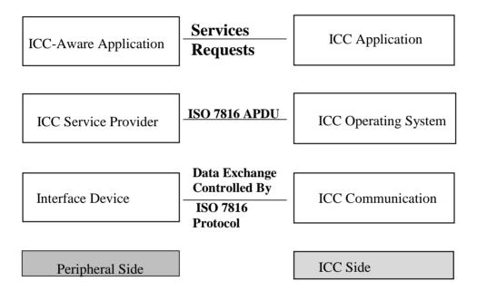
Figure 2-2. ICC/PC communication layers
